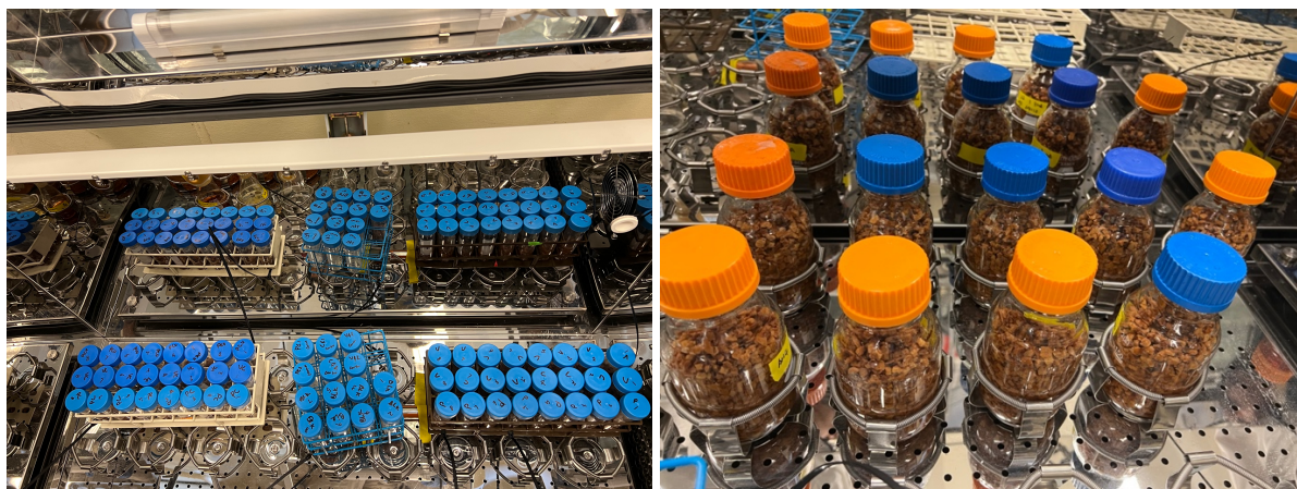
Figure 5. 3. Enzymatic hydrolysis of residual almond hull solids in incubator shaker. left: small scale (20 mL); right: large scale (200 mL)
