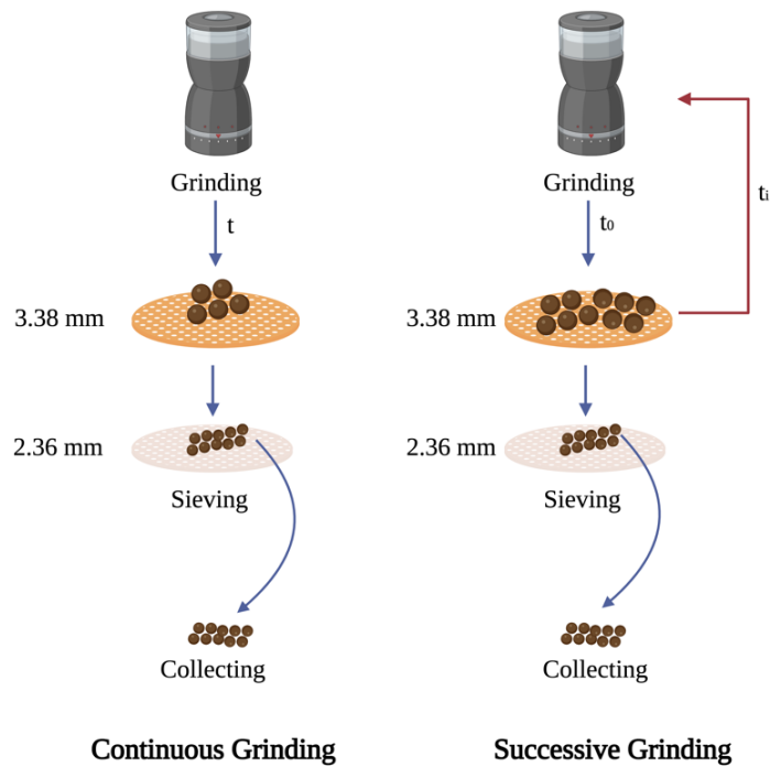
Figure 2. 3. Description of continuous and successive grinding processes
