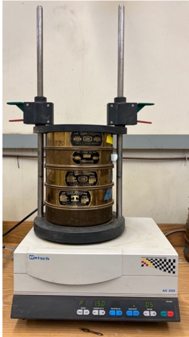
Figure 2. 2. Sieve shaker used to separate almond hulls with different size
