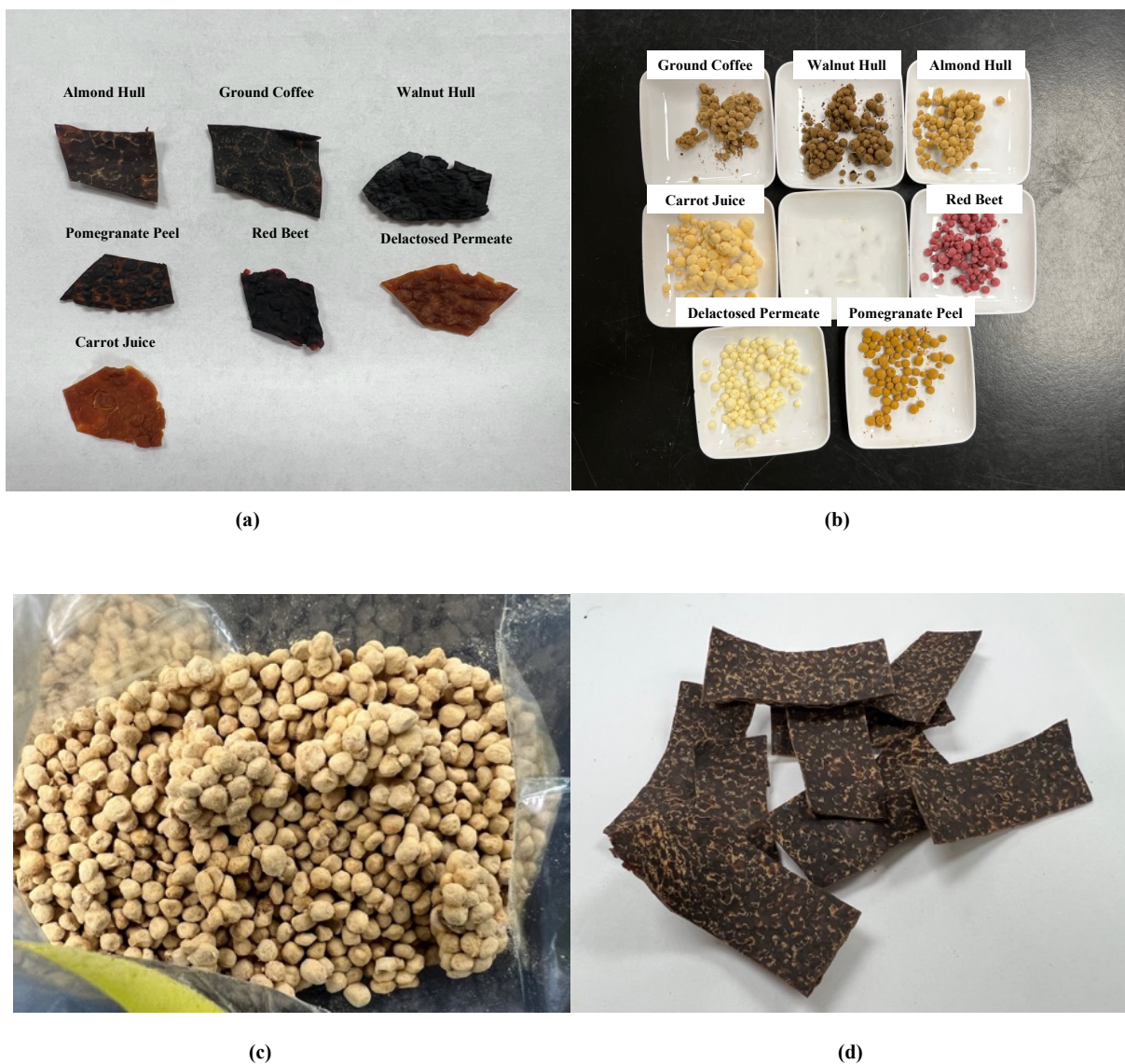
Figure 7. 15. Dried fungal biomass cultivated from natural materials by freeze drying or hot air drying. (a) hot air dried fungal biomass from natural materials; (b) freeze dried fungal biomass from natural materials; (c) freeze dried fungal biomass from almond hulls; (d) hot air-dried fungal biomass from almond hulls
