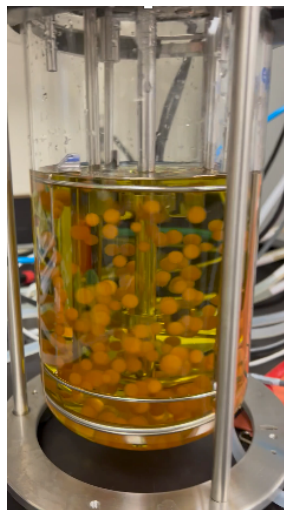
Figure 4. 19. Mixing intensity testing by precultured pellets
