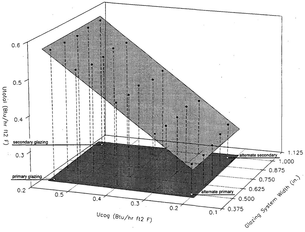
Figure 3. Total window U-value as a function of glazing thickness and center-of-glass U-value. By definition of WINDOW4's linear interpolation, all total window U-values calculated with the four point simulation method and based on valid glazing configurations will lie on the lightly shaded plane of total window U-Values.
