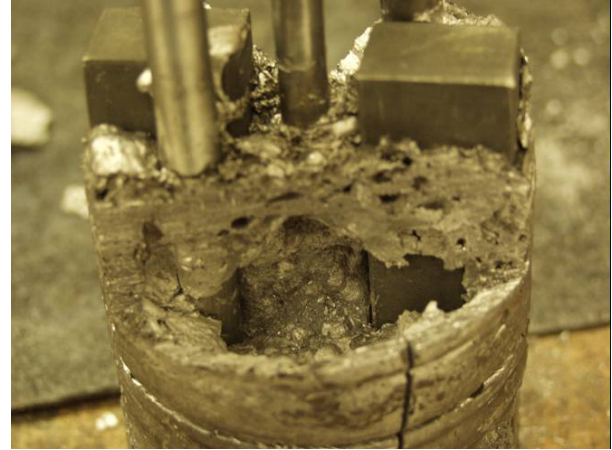
Figure 12. Gas pocket formed in the liquid metal around the propeller. This state was solidified by liquid nitrogen.
