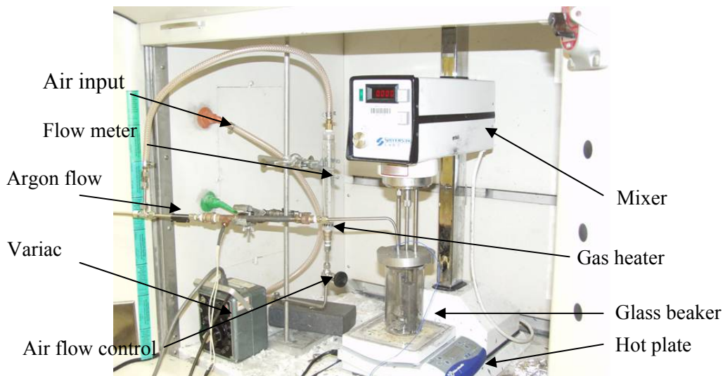
Figure 10. Experimental setup to control the quantity of oxygen in the gas flow
