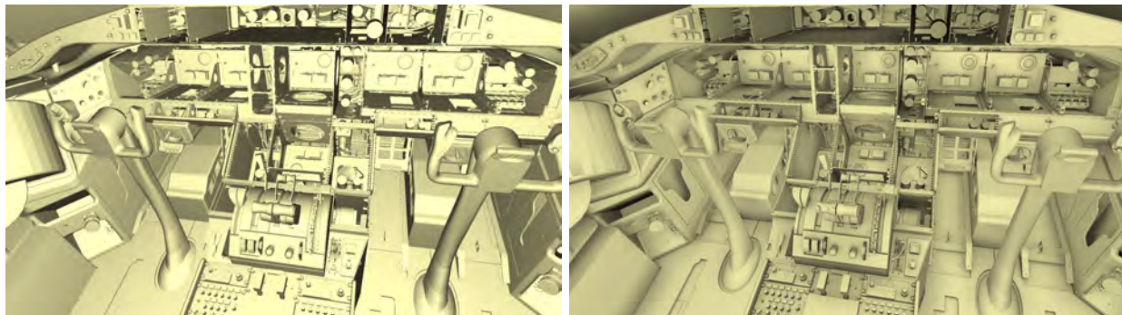
Figure 5: On 60 nodes, the 259M triangle Boeing data set using HD resolution can be ray cast (left image) at 96fps if all 15,637MB of triangle and acceleration structure data are replicated on each node and at 77fps if DC is used to store only 1,955MB of data and cache per node. Using 36 ambient occlusion rays per pixel (right image) the system achieves 1.46fps. Image source: Ize et al. [16].
