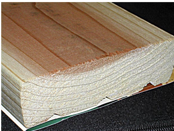
Figure 1. The sapwood of any species is not very durable. Color can often help distinguish the heartwood and sapwood of a species. In this redwood ( Sequoia sempervirens ) board, the reddish wood on top is the heartwood and the white portion is sapwood.
