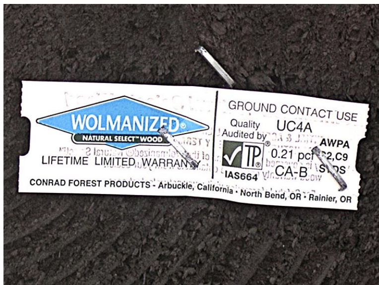
Figure 6. Typical tag on pressure treated lumber, in this case indicating the preservative chemical is Copper Azole, and that the lumber has been treated for a ground contact application. “TP” is a quality control indicator; “UC4A” refers to the lumber’s application (“use category”), and is in this case is somewhat redundant with the “ground contact use” statement.
