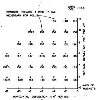
140 MA, EQUIV. TO 1.52 x 10 GAUSS-IN OR 7 MEV PROTON
