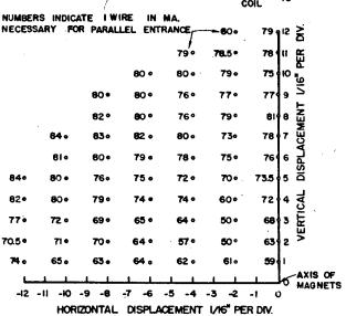
80 MA EQUIV. TO 3.37 X 105 GAUSS-IN OR 35 MEV PROTON
