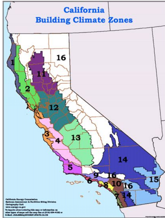
Figure 3.2: California Energy Commission building climate zones
