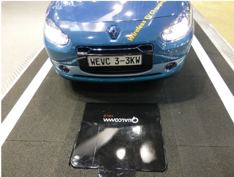
Figure 6. Qualcomm Halo Wireless Charging
