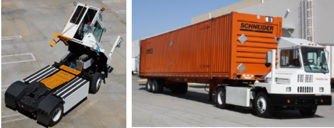
Figure 23. TransPower Demonstration Vehicles: Electric Yard Tractor, attached to trailer (right)
