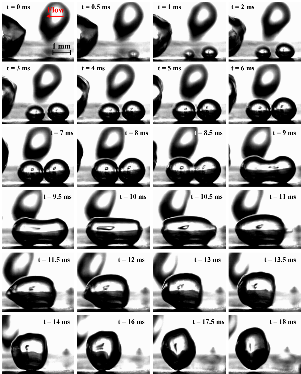
Figure 4.31 Two-bubble merger growth cycle, for vertical aluminum surface, U_{\text{bulk}} = 0.1 m/s, \Delta T_w = 5.5 °C, \Delta T_{\text{sub}} = 0.4 °C and x_{\text{cav}} = 1.2 mm.
