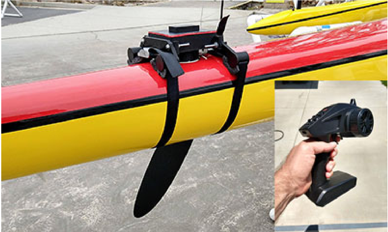
Figure 4.5: A close-up of version two of the CoOP system mounted to the rudder assembly and the transmitter used to control the rudder (right corner).
