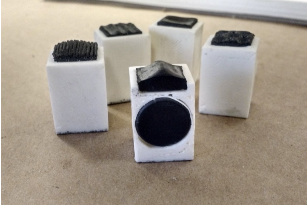
Figure 3.2: The physical icons used in the Tangible Desktop (see Figure 3.1). Each icon has an RFID tag embedded inside and a tactilely distinct rubber crown.
