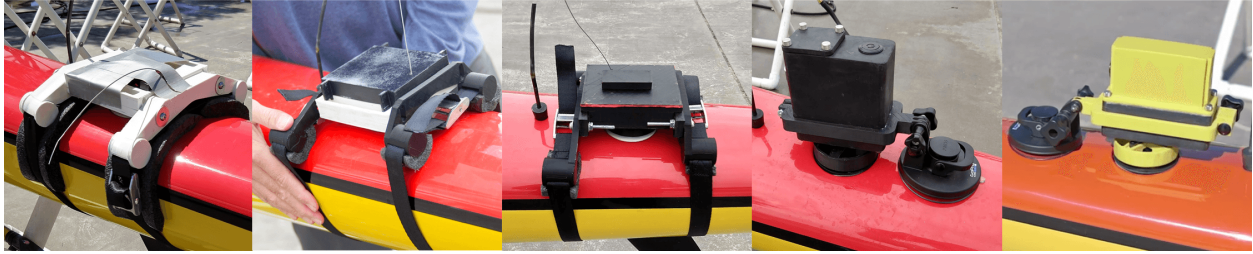
Figure 4.6: The design evolution of the CoOP system in order of iteration from left to right. Early iterations of CoOP version 1 are depicted in the first three pictures from the left, followed by versions 2 and 3.
