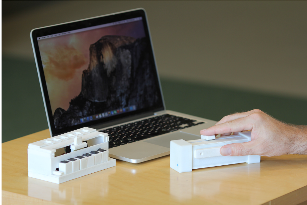
Figure 3.1: A picture of the Tangible Desktop in its standard arrangement. The Tangible Taskbar sits to the left of the laptop while a user engages with the thumb of the Tangible Scrollbar.
