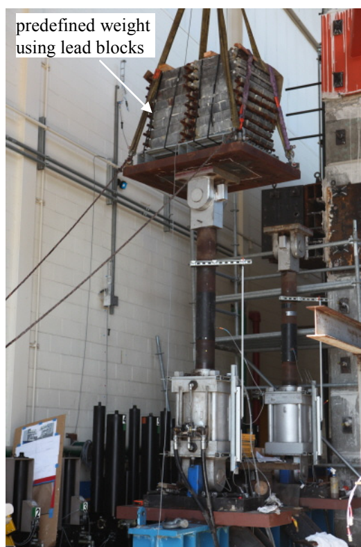
Figure IV.13 Calibration of load cell of the column axial loading actuator.
