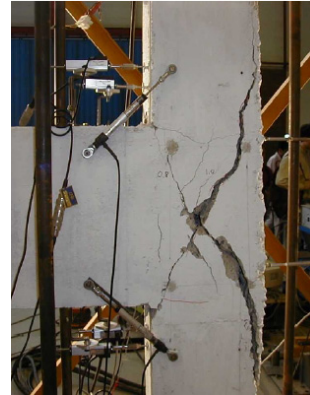
(b) Two relative beam-column deformations (Pampanin et al., 2003)
