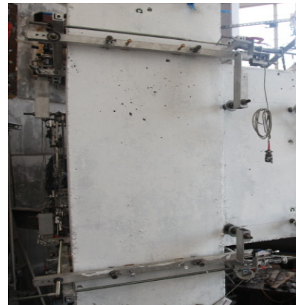
Figure IV.17 Instrumentation for rotation at the beam-joint interface.
