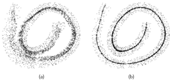
Figure 27: Curve reconstruction using MLS (a) and Lee's approach (b). The pluses are the input points and the squares are the projected points. From [Lee 2000].
