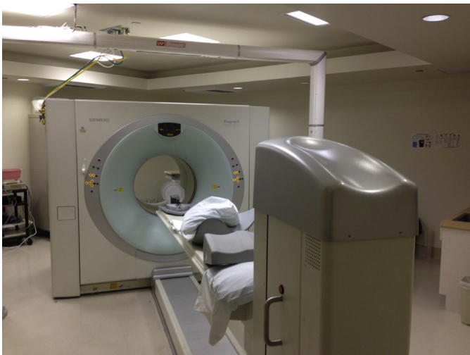
Fig. 6. A cardiac PET scanner (Siemens Biograph PET-CT scanner [Siemens Medical Solutions, Malvern, PA]).
