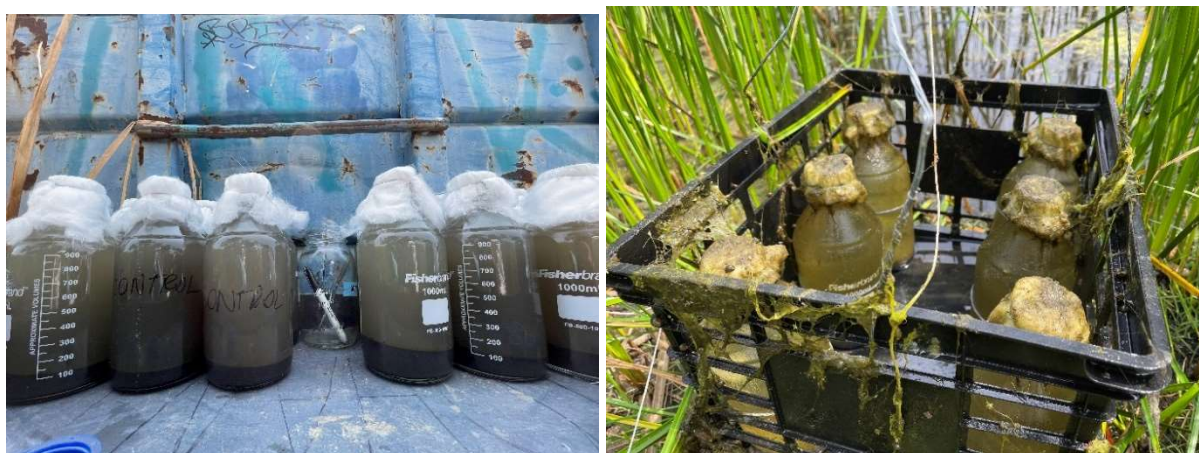
Figure 5.1 – Picture of the experimental bottles that were submerged in the Ballona Wetland for 130 days. 6 identical bottles were used for the control experiment, and other 6 identical bottles were used for the experiment with wetland residues. The containers (control and wildfire) were submerged next to each other in the wetland.
