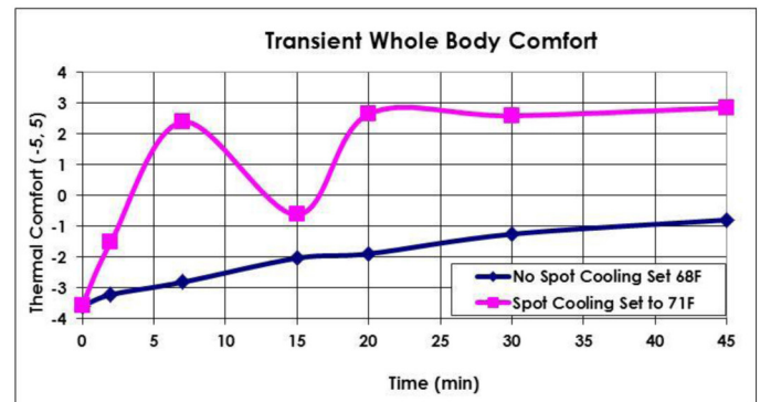
Figure 34. Thermal Comfort Rating during Soak and Cool-Down at the Ambient Condition of 37.8^{\circ}\text{C}\times 40\%\times 1000\text{W}/\text{m}^2
