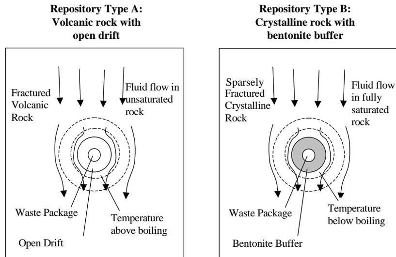
Fig. 1. Schematic showing the two repository scenarios (vertical cross section)
