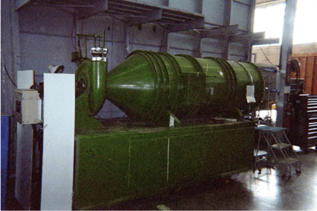
Figure 2 Airflow measurement apparatus at Energy System Laboratory – air exit at left – furnace or blower to be tested mounts on the right
