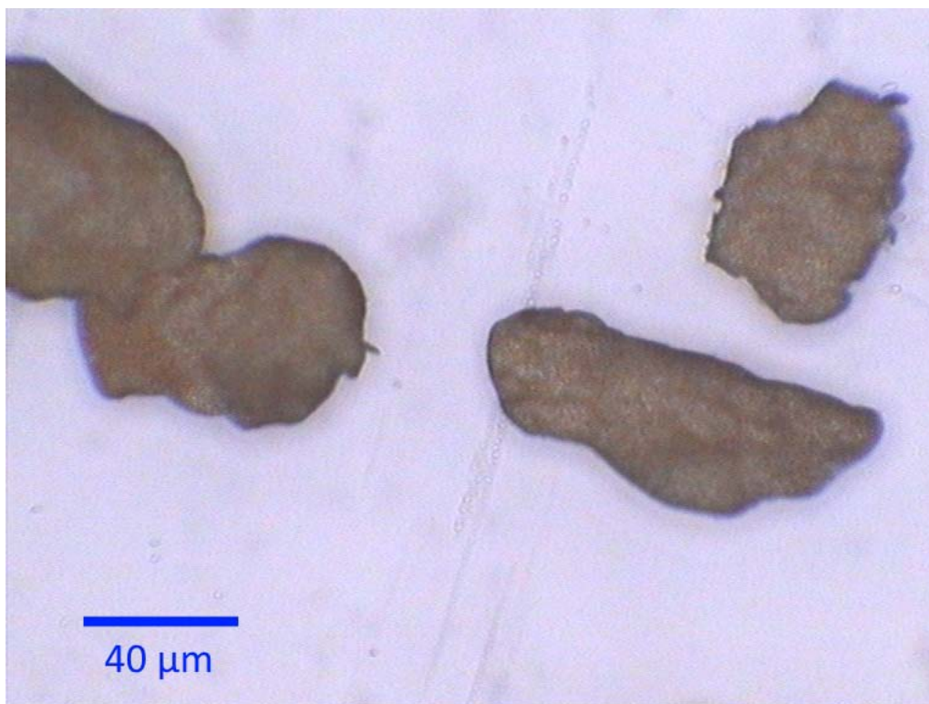
Figure 5.4: Microscopy image of synthesized goethite particles from the 75-150 \mu\text{m} size fraction.
