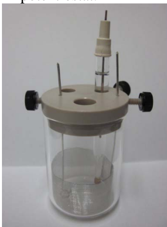
Figure C 3: A picture of the electrochemical cell used in this work that shows the Ag/AgCl reference electrode (right side), platinum mesh working electrode, and Pt wire counter electrode (left side).
