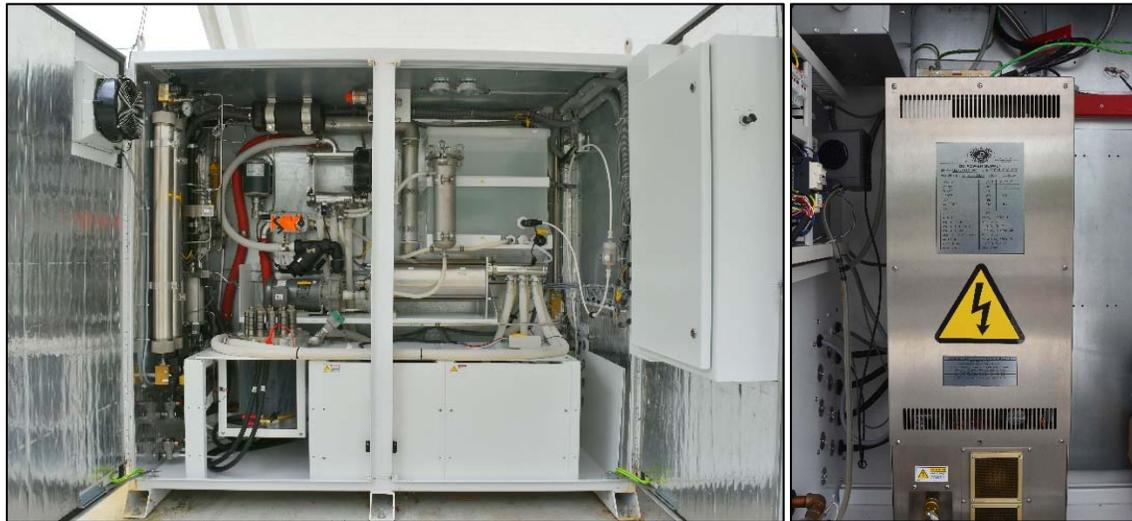
*Figure 4. C10 electrolyzer system. Fluids cabinet containing mechanical systems and cell stack on the left, electrical cabinet containing the power electronics on the right.*
