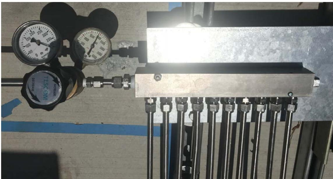
*Figure 89. Pressure regulator and cylinder manifold used in high throughput hydrogen testing.*
