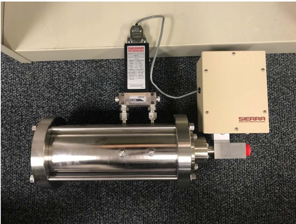
*Figure 87. Sierra Hi-Trak 840 mass flow controller utilized in high throughput hydrogen injection testing.*
