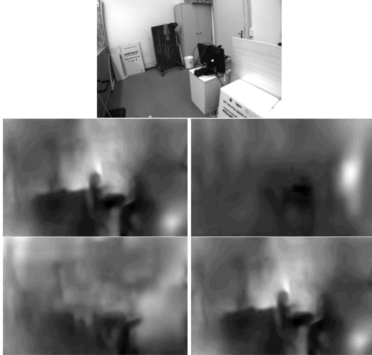
**Figure 4.15:** Depth maps for a random frame in V1 02 sequence. Top row: original frame. Middle row: learner-mh (left) and learner-v1 (right). Bottom row: learner-mhv1 (left) and learner-euroc (right). Interestingly, none of the models are able to produce a decent depth map for the frame.
