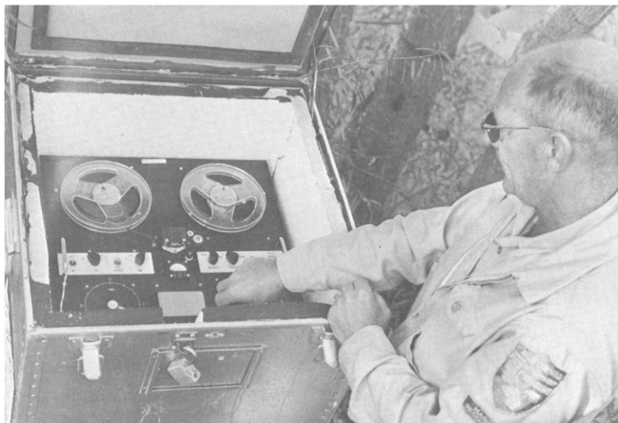
FIGURE 10. Tape recorder type of stationary sonic tag monitor used in 1965–1967; note insulated housing box. Photograph by Wm. F. Van Woert.
