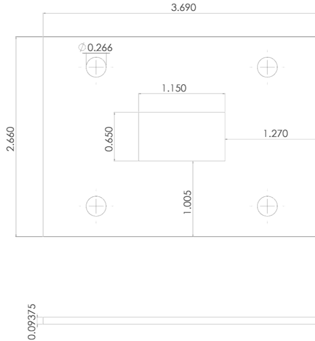
Figure E-2. Schematic of the membrane cell spacer made with white Delrin acetal resin having dimensions of 2.66" (width) x 3.69 (length) x 0.09375 (height) (Note: all dimensions are in inches).
