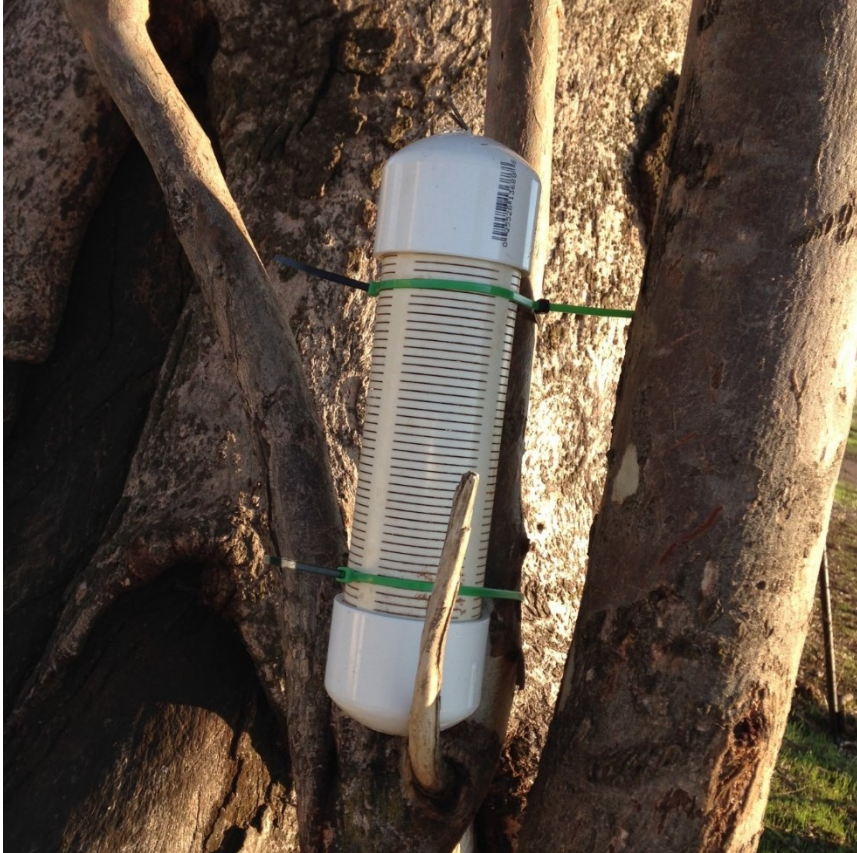
Figure 14 Model Barologger Edge (Solinst, Georgetown, Ontario, Canada) placed inside a slotted PVC pipe and tied to a tree.
