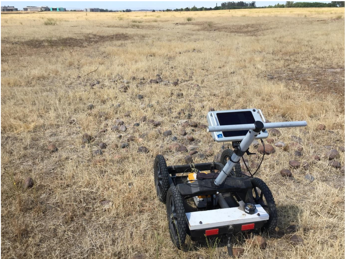
Figure 8 MALÅ Geoscience X3M ground–penetrating radar (GPR) system (MALÅ Geoscience, Malå, Lapland, Sweden) connected to an 800 MHz shielded antenna was mounted on a cart and used to survey the depth of changes in soil horizon texture.
