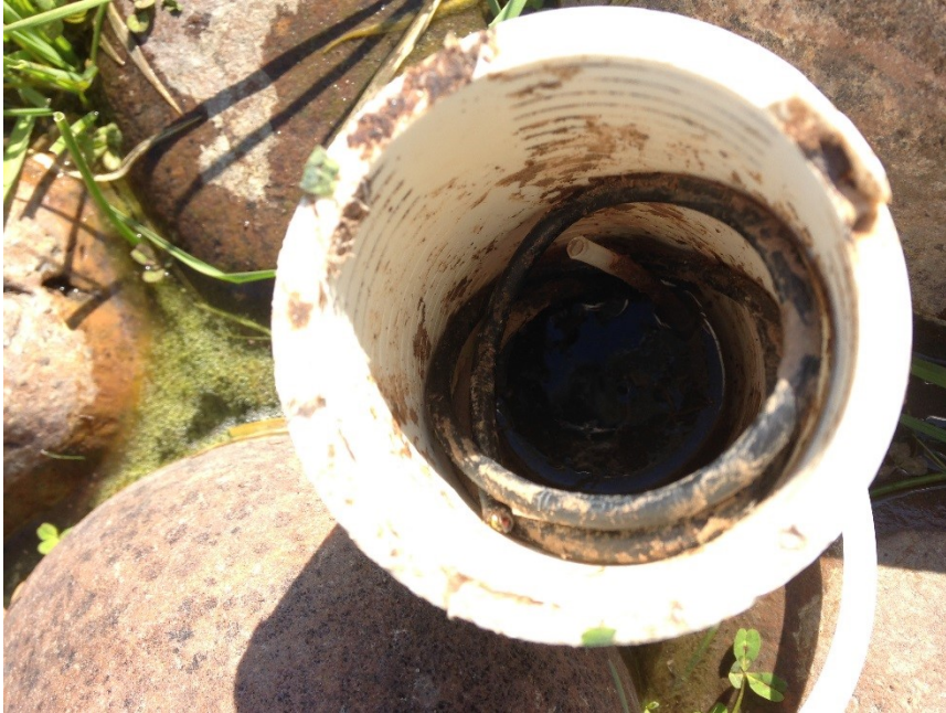
Figure 9 Inside a monitoring well. Model 3001 Junior M5 Levellogger (Solinst, Georgetown, Ontario, Canada) and Model 1911-B.5 remote soil water sampler (SoilMoisture, Santa Barbara, California, USA) deployed inside a two-inch slotted PVC pipe.
