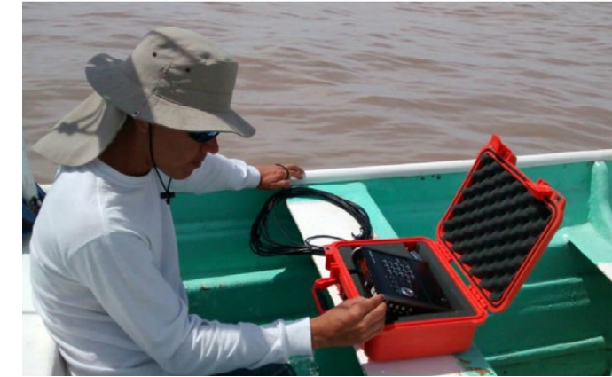
Figure 15. Portable hydrophone connected to a recorder. The cabled hydrophone is lowered off the side of the boat to record underwater sound, while the recorder saves the files for future processing. This configuration is appropriate for mobile surveys conducted off a boat.
