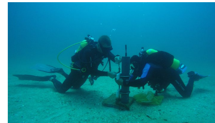
Figure 16. Self-contained hydrophone being deployed. These combined hydrophone and recorders enable to the collection of sound recordings over long periods of times at fixed locations.
