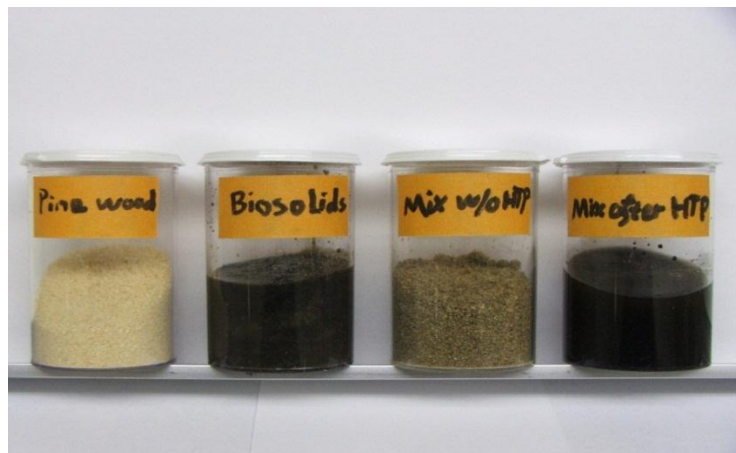
Figure 2.2 Untreated and HTP treated biomass and biosolid mixture samples
