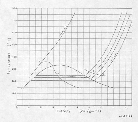
Fig. 32. Temperature - entropy diagram of hydrogen, showing control system operation of the hydrogen refrigerator for the Berkeley 72-inch bubble chamber.
