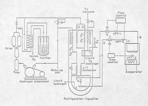
Fig. 31. Schematic flow diagram of hydrogen refrigeration system for the Berkeley 72-inch bubble chamber.
