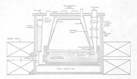
Fig. 18. Longitudinal cross section of the Berkeley 72-inch bubble chamber. (The direction of the magnetic field is vertical.)
