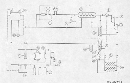
Fig. 37. Flow diagram of the CERN 2-meter hydrogen refrigeration plant.
