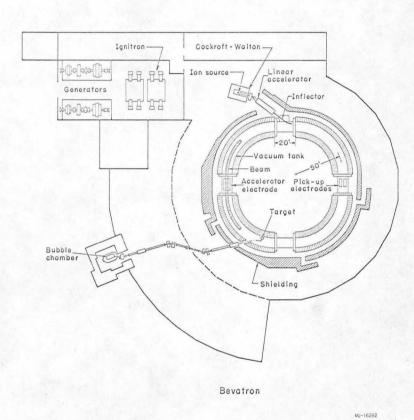
Fig. 5. Particle path from the Bevatron, through the beam path, and into the 72-inch bubble chamber (Berkeley).
