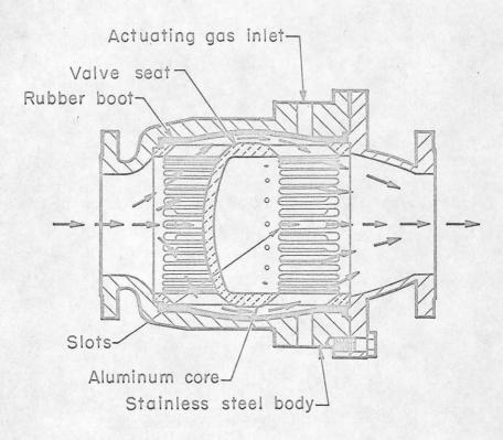
Fig. 28. Grove-type boot valve shown in section.
