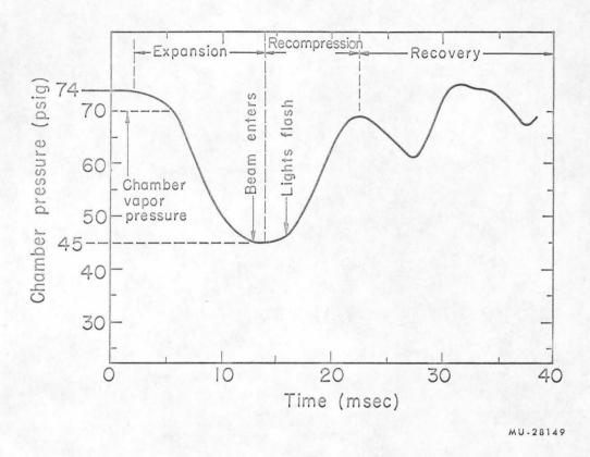
Fig. 13. Typical expansion-recompression cycle for a liquid-hydrogen bubble chamber.
