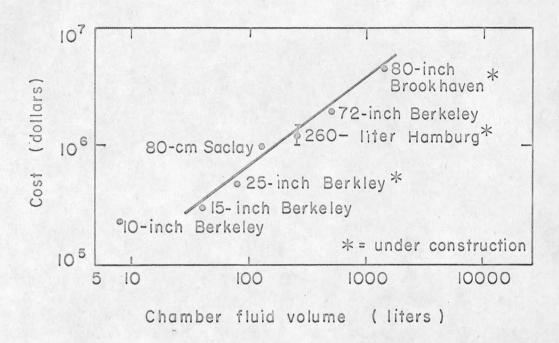
Fig. 40. Approximate cost to build a bubble chamber, as a function of chamber volume.
