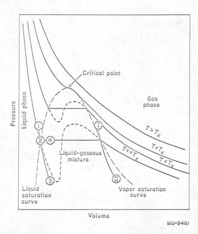
Fig. 2. Pressure-volume plot of representative expansion curves for a real gas, showing zones of operation for bubble chambers (1 2 3 4) and cloud chambers (I).
