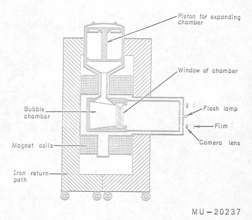
Fig. 16. Transverse cross section of 80-inch Brookhaven liquid hydrogen bubble chamber.
