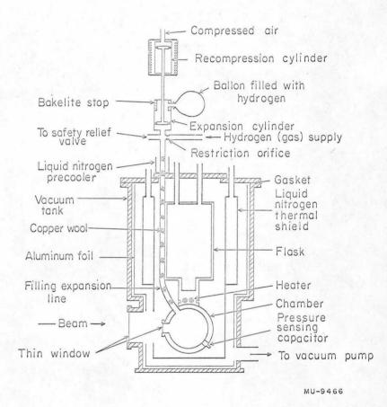
Fig. 8. Cross section of Berkeley 4-inch liquid hydrogen bubble chamber.
