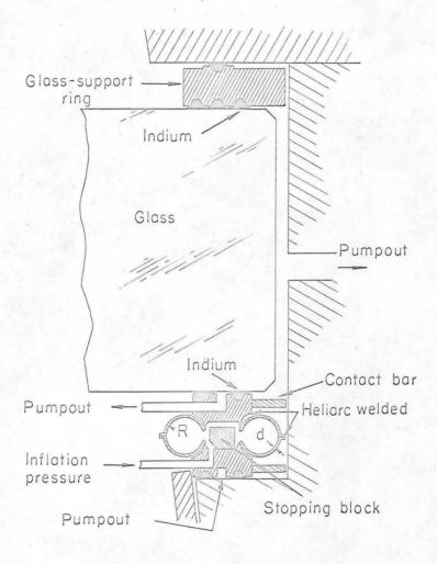
Fig. 24. Cross section of the inflatable gasket and related parts for the Berkeley 72-inch bubble chamber.
