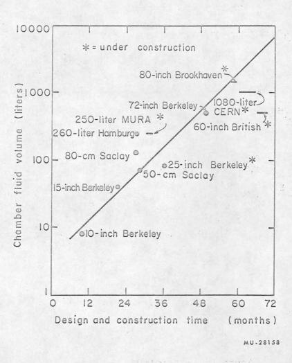
Fig. 39. Approximate total time required to build a bubble chamber (from conception to operation) as a function of chamber volume.
