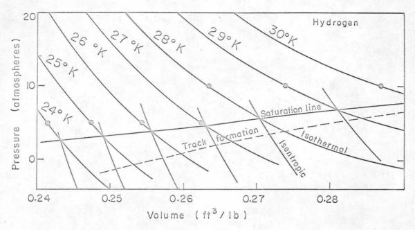
Fig. 14. Isothermal and isentropic pressure-volume curves for hydrogen. These curves were computed below the vapor-pressure line by
