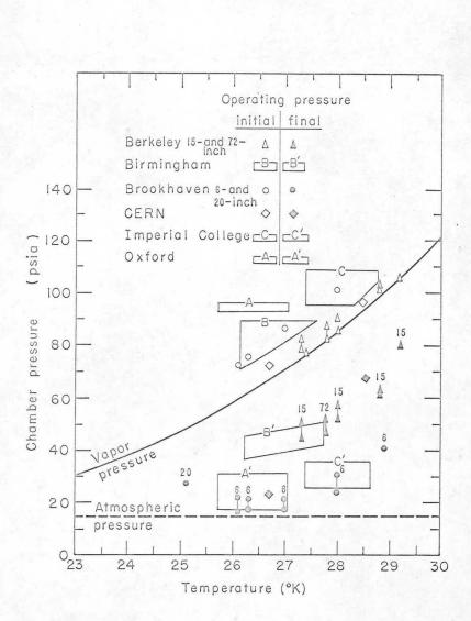
Fig. 12. Normal range of operating temperature and pressure for liquid hydrogen bubble chambers.
