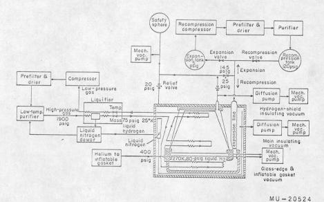
Fig. 25. Simplified schematic of expansion, refrigeration, vacuum, and safety-vent systems for the Berkeley 72-inch bubble chamber.
