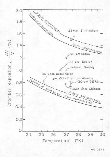
Fig. 15. Change in volume of several liquid hydrogen bubble chambers during the expansion cycle. Chambers with the most efficient expansion systems have lower expansion ratios,  $\Delta V/V$ , and operate near the isentropic expansion curve.
