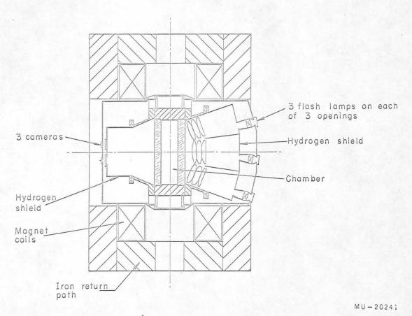
Fig. 17. Plan view of 60-inch British National liquid hydrogen bubble chamber.
