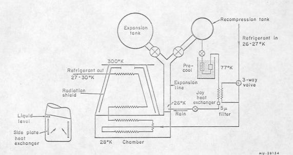
Fig. 27. Schematic representation of refrigeration circuit for the Berkeley 72-inch bubble chamber, showing how liquid hydrogen is introduced into the expansion line at the liquid - gas interface.
