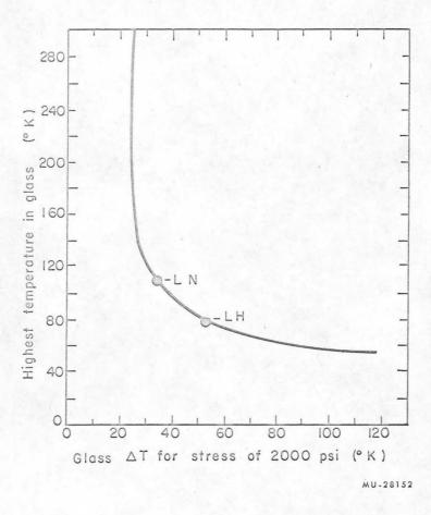
Fig. 23. The allowable temperature difference, ΔT, of the chamber glass to limit the thermal stress to 2000 psi. The points marked LN and LH give the highest temperatures at which LN and LH can make contact with the glass and not stress the glass more than 2000 psi.
