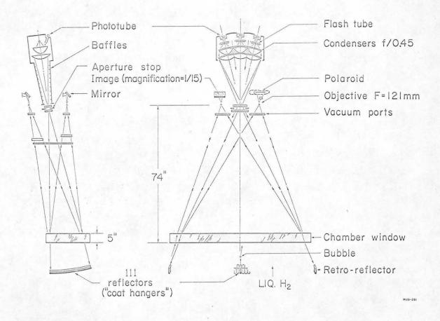
Fig. 4. Optical system of the Berkeley 72-inch bubble chamber.
