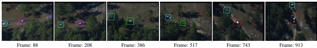
Fig. 15: Multi-target tracking results of a scene (frame no. 88, 208, 386, 517, 743, and 913) of VIVID aerial video dataset. Different targets are given different colors and IDs.
