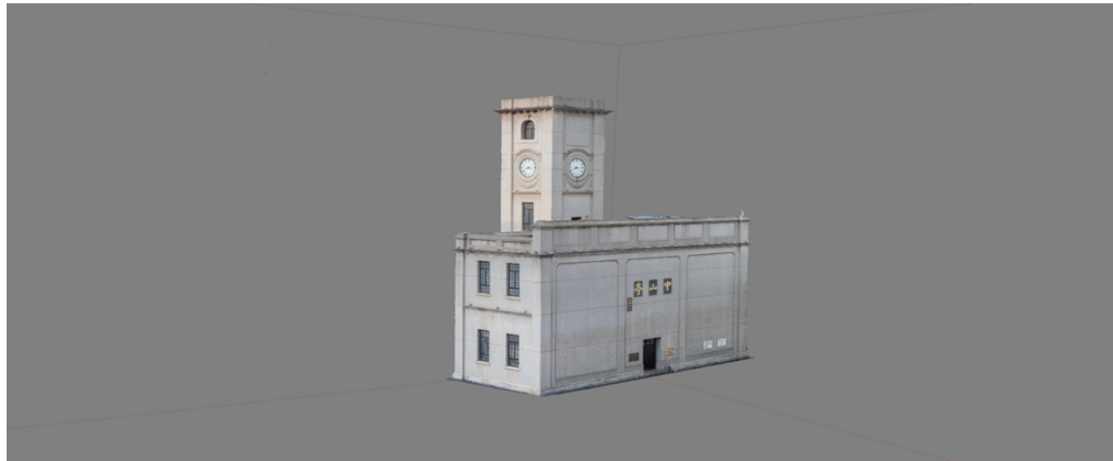
Figure 7 Dense cloud generated by Agisoft Metashape based on the images before generating mesh. Image courtesy of the author.
