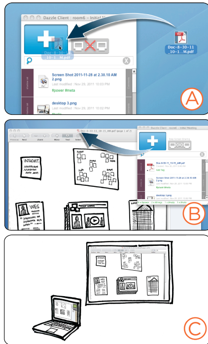
Figure 28: To bring a file to others' attention, the participant drags that file on to the drop target (A). This opens the file locally on that person's computer (B) as well as initiates screen sharing with a public display (C).
