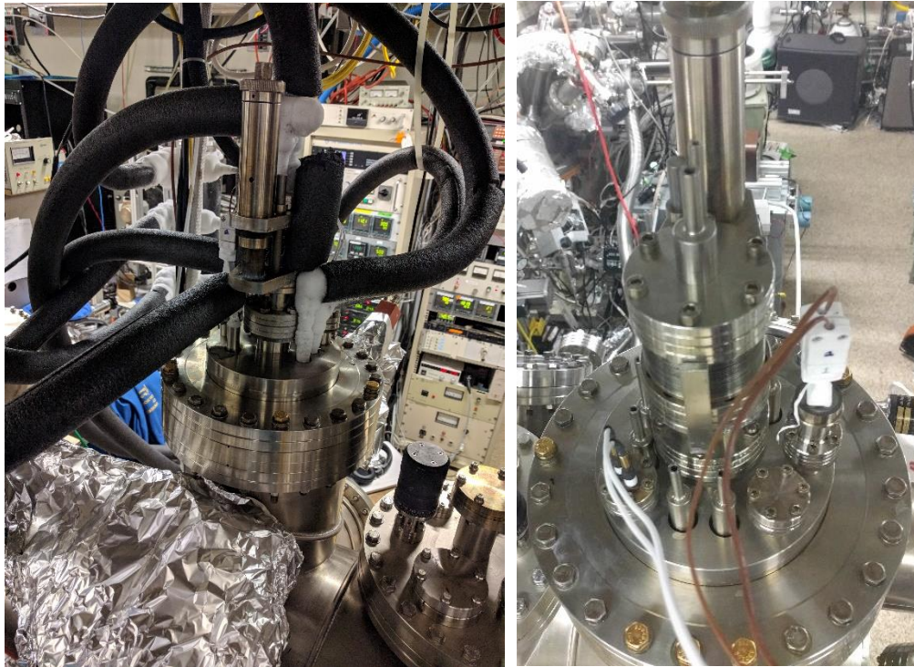
Figure B.17 The right panel shows the cryogenic sample stage manufactured by VG Semicon, without any plumbing attached to it. The left panel shows the new plumbing attached to the stage with thermal insulation (black). During operation ice builds up on joints not covered by insulation.
