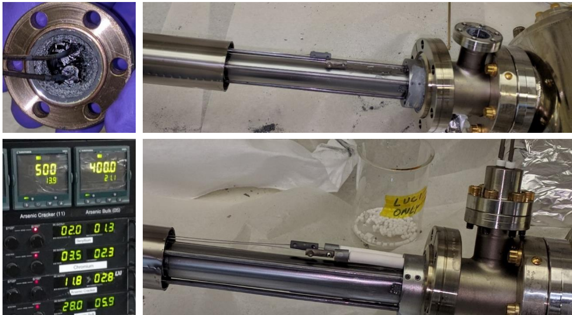
Figure B.6 The left-top picture shows the leaking thermocouple on the cracking zone of the Arsenic cell. The thermocouple was also not operational and was reading the temperature of the chamber wall, which could be attributed to the excessive amount of Arsenic shorting the two terminals. Right-top: Cracking zone with thermocouple removed. Right-bottom: Cracking zone with new thermocouple installed with ceramics (white) encasing the thermocouple lines. Left-bottom: Cracker thermocouple in operation reading 500^\circ\text{C} .
