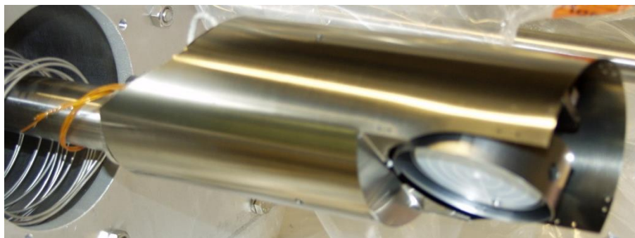
Figure B.7 The top panel shows the new manipulator from UHV-Design with a gold coated glass tube for back-side illumination of the sample. The center panel shows the Kapton lines on the manipulator. The bottom panel shows the old shield to protect manipulator parts from III-V flux.
