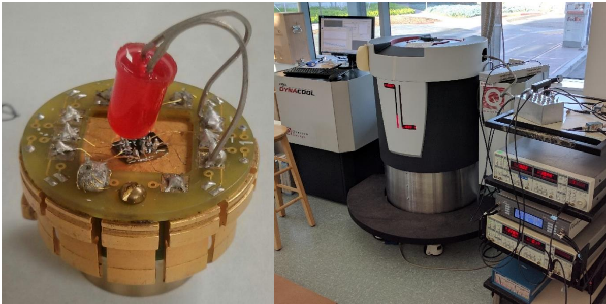
Figure 3.5 The left panels shows a PPMS puck used to measure Hall bars fabricated of quantum well structures. Hall bars on the semiconductor are connected with In:Sn solder, via gold wires, to another blob of In:Sn solder on the PPMS puck. In samples requiring external illumination, a generic red colored LED is installed on two pins of the puck. The LED was operated at 10mA constant current, and limited the base temperature of the PPMS to 4-10K. Once the LED was turned off a base temperature of <2K could be achieved. On the right is a typical measurement setup showing the Quantum Design DynaCool cryogen free PPMS. The puck shown on the left is inserted in the PPMS and cooled to ~1.8K and measured at fields up to 9 Tesla using AC lock-in technique. Lock-in amplifiers and a GPIB ground isolator are pictured in the instrument cart on the right.
