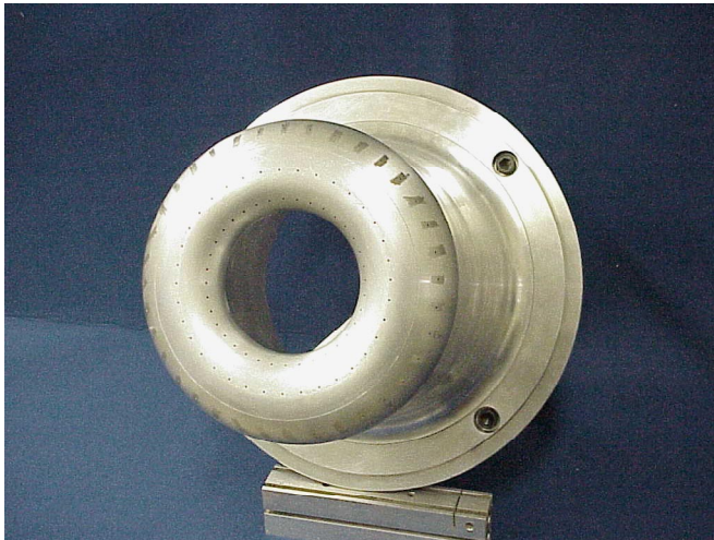
Figure 13: Inner body detail: fuel injection points
