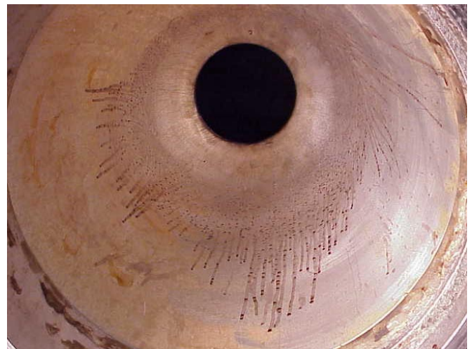
Figure 18: Surface Flow Indicating Fluid traces; Generation 1 Novel Premixer Outer Body.
