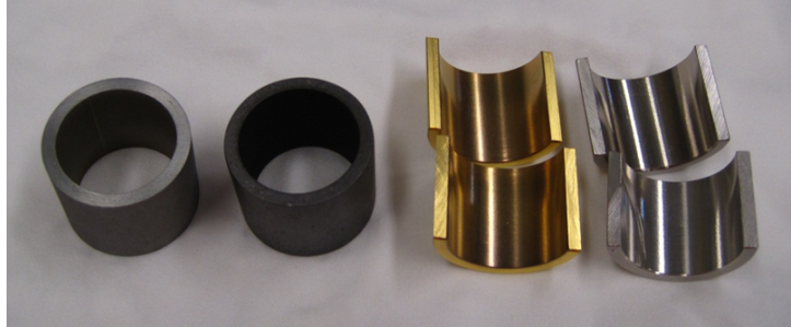
Figure 2.9: Molybdenum, graphite, gold, platinum anode pieces.
