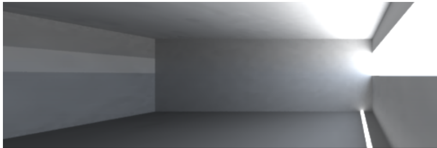
Figure 8. Prototypical Clerestory Office simulation using holographic glazing with 50° acceptance and 55.7° diffraction angles for Noon on June 21 (direct solar radiation is at 67.6°).
