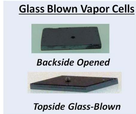
(b) Fabricated and gas filled vapor cells
