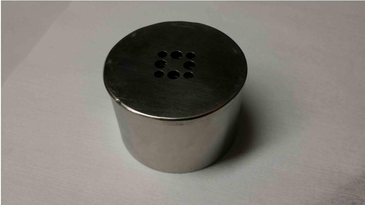
Figure 3.39: Manufactured 5 layer magnetic shield
