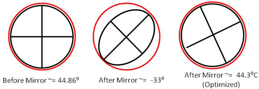
Figure 3.19: Polarization changes due to dielectric mirrors
