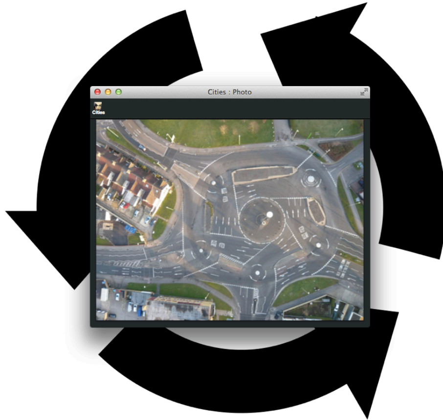
Figure 82 Screenshot configuration by the author: (middle) a contemporary aerial photograph of Swindon’s Magic Roundabout, designed by Frank Blackmore, the same engineer who came up with the priority rules that define the “modern roundabout.” (source: Google Images).
