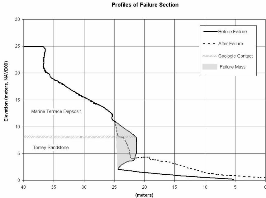
Figure 8. Before and after profiles of the Solana Beach cliff failure.
