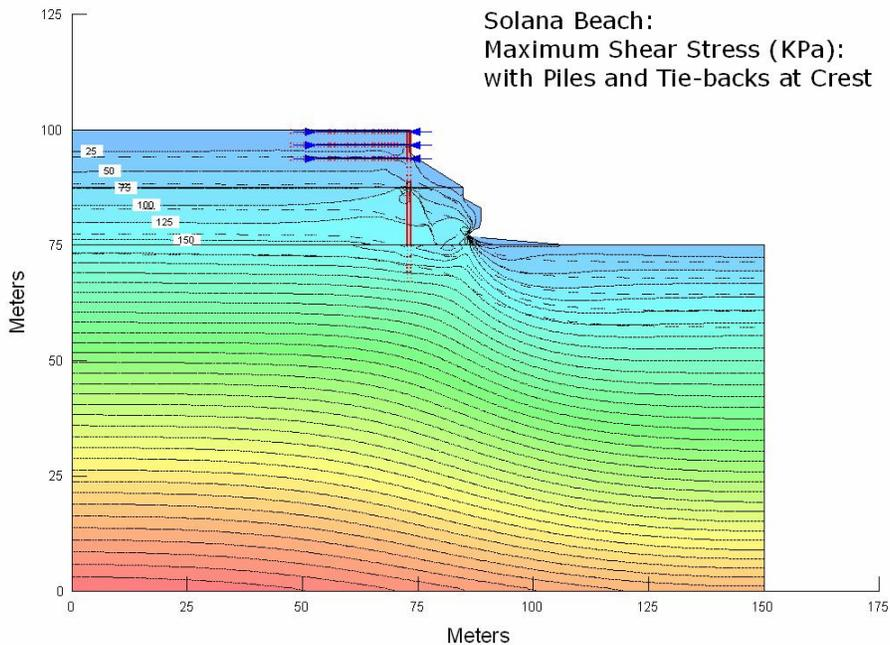
Figure 10. Theoretical stress distribution with erosion control measures.
