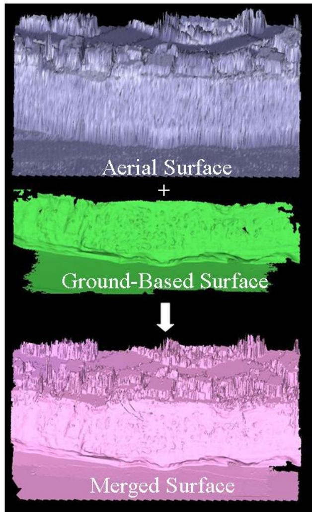
Figure 11. Merging aerial and ground-based LIDAR surfaces.
