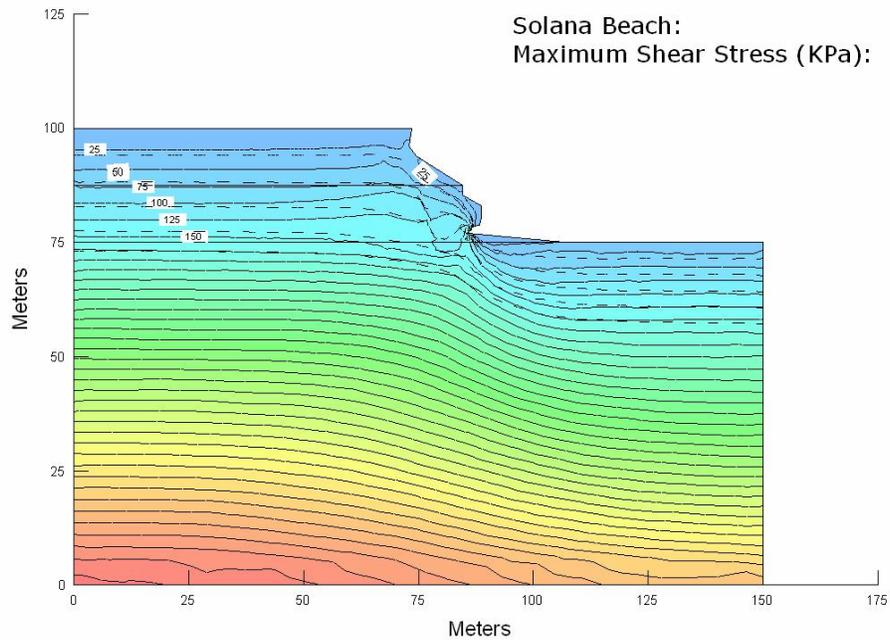
Figure 9. Theoretical shear stresses prior to the Solana Beach failure.
