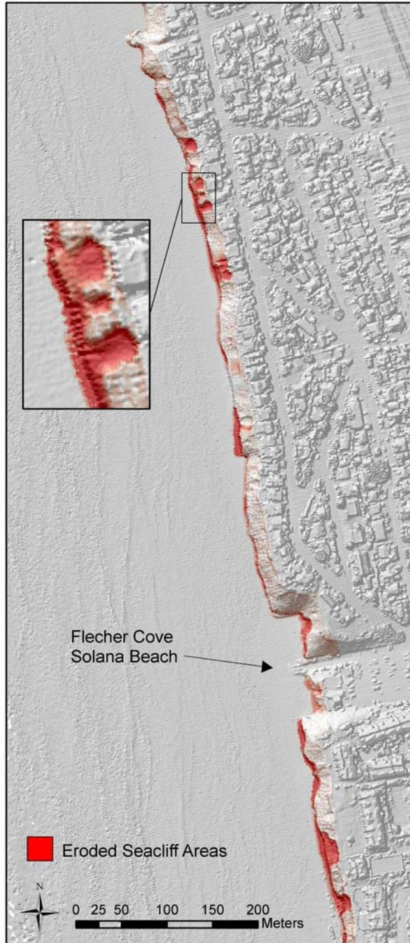
Figure 2. Areas of seacliff erosion in Solana Beach from April 1998 to April 2004.
