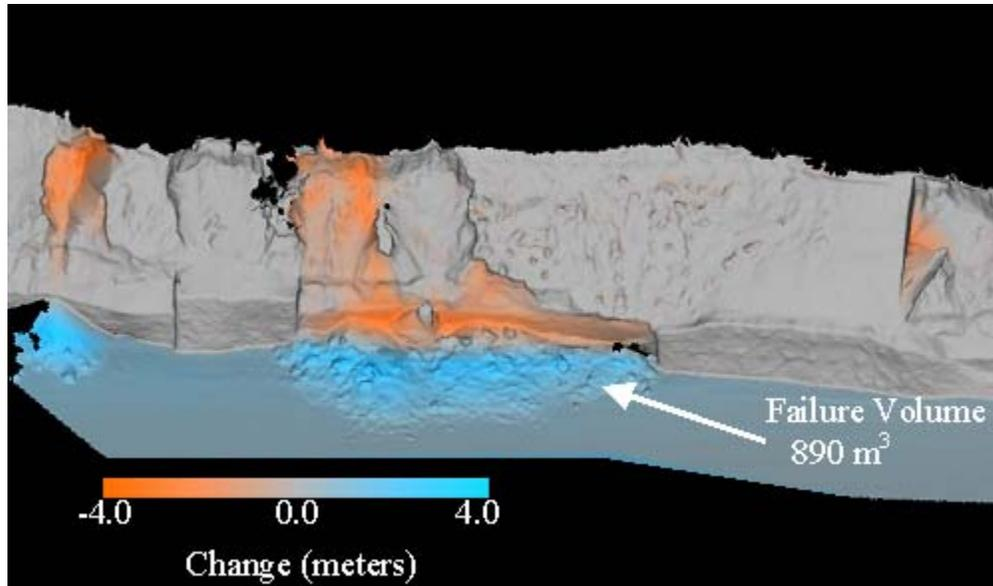
Figure 7. Major seacliff failure in Solana Beach.
