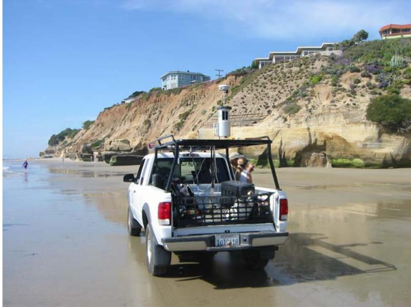
Figure 5. Mobile ground-based LIDAR setup.
