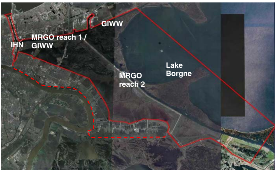
Fig. 2 FINEL model computational domain outlined in solid line. Urban area bounded on west with dashed line
