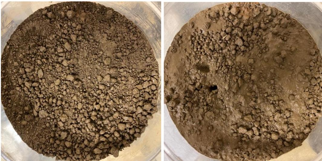
Figure: Photograph of the top view of the soil column before (left) and after (right) running the experiment for T3.
