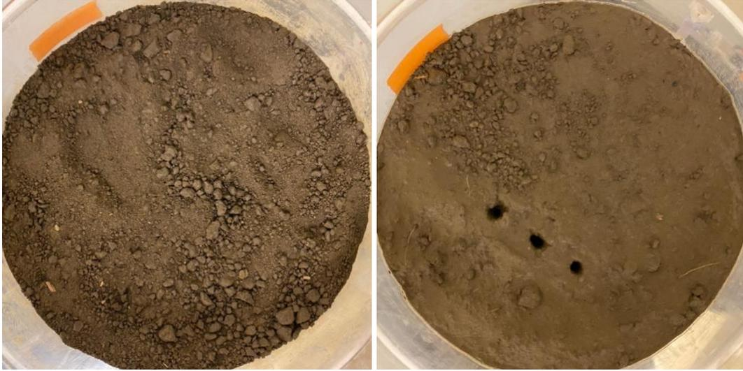
Figure: Photograph of the top view of the soil column before (left) and after (right) running the experiment for T4.
