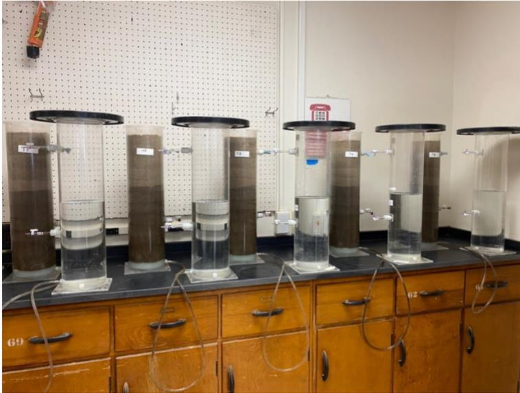
Figure: Bottom-up pre-saturation of the soil column with tap water before running the infiltration experiment.
