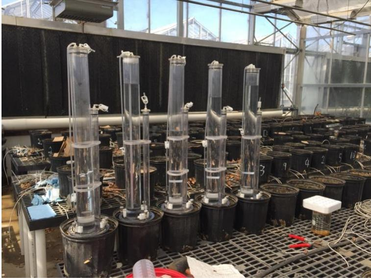
Figure: Infiltration experiment conducted over the soil in pots after terminating the greenhouse experiment. The results are presented in Chapter 3 in Figure 3.5.
