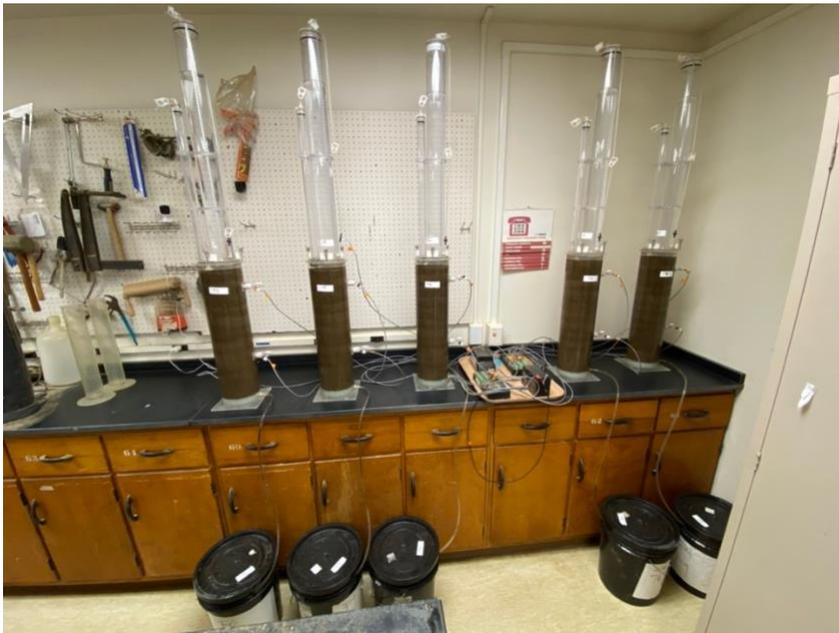
Figure: Running the infiltration experiment using the wooding infiltrometer and collection of the drainage water into the buckets that are in the ground.
