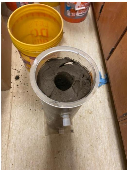
Figure: Sampling from the soil columns by depth using augur core sampler after conducting the infiltration experiment. The results of the clay dispersion by depth are shown in Chapter 2 Figure 2.7.
