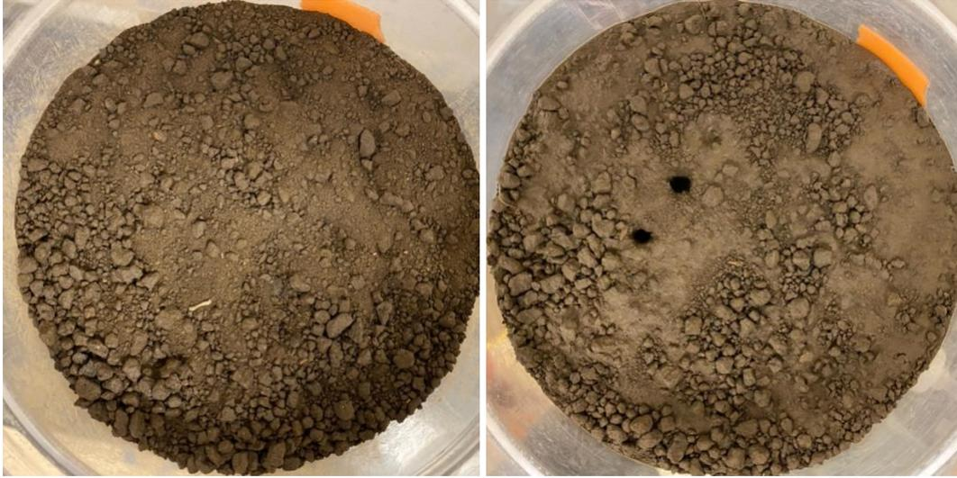
Figure: Photograph of the top view of the soil column before (left) and after (right) running the experiment for T0.
