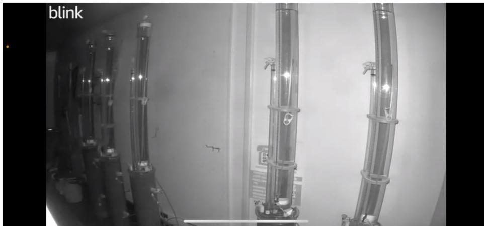
Figure: Screenshot from the blink APP coupled with Blink Camera to live monitor the water level in the wooding infiltrometer to make sure that water does run out. The camera turns to night vision when the lab lights are off.
