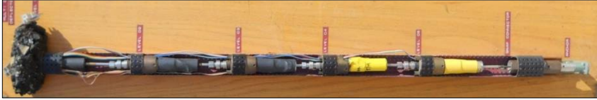
Figure 4.3: A model multi-depth deflectometer (MDD), showing five modules.
