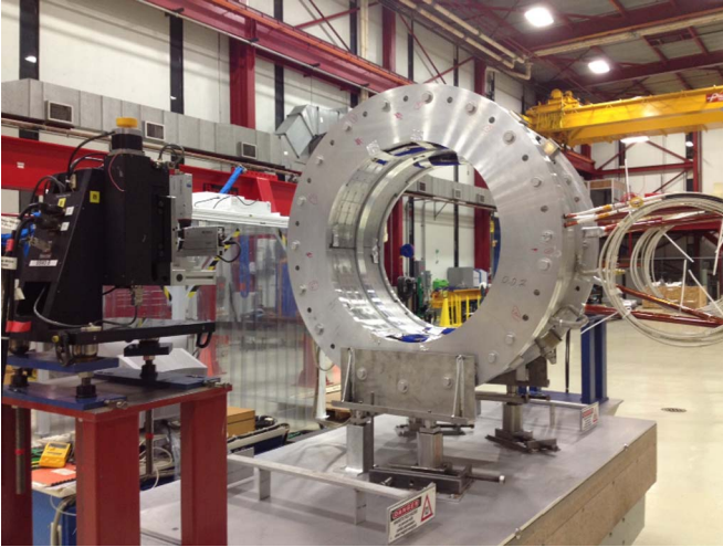
Fig. 3. TS prototype on the vibrating stretched-wire station.
