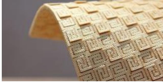
Figure 38. Plywood sheet laser cut to form a flexible geometry (koFAKTORlab, 2013)
