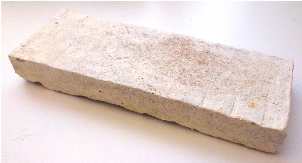
Figure 41. De-molded block of mycelium composite, showing white mycelium surface growth
