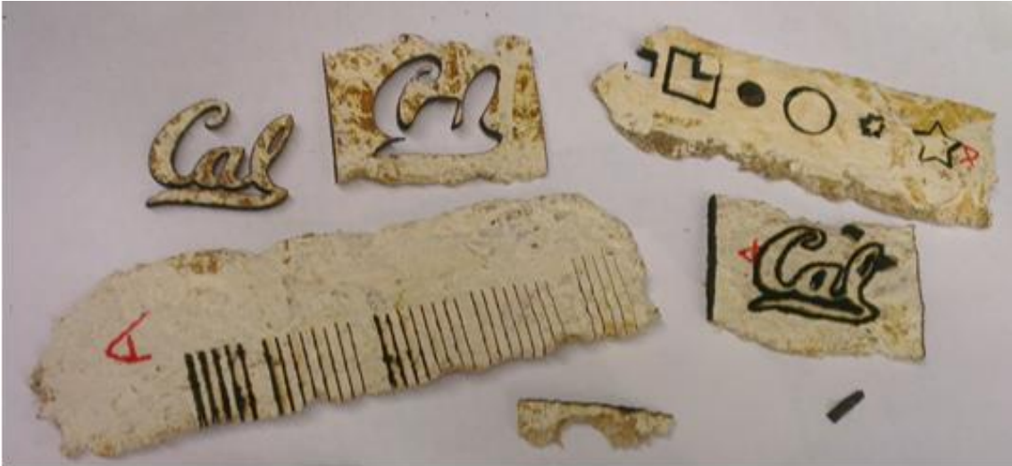
Figure 37. Examples of laser cut mycelium materials created during laser cutting testing
