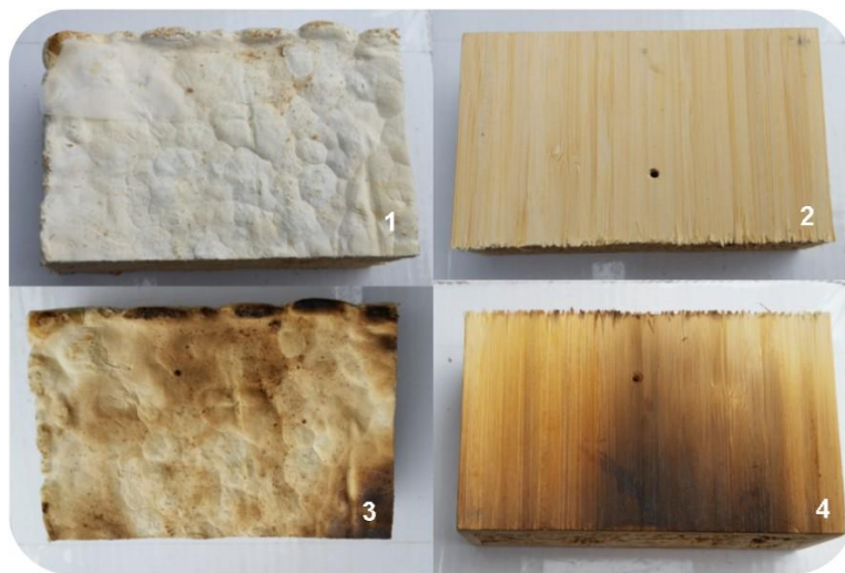
Figure 18. Material types L and J before exposure to hot surface in 1 and 2 respectively, and after in 3 and 4.
