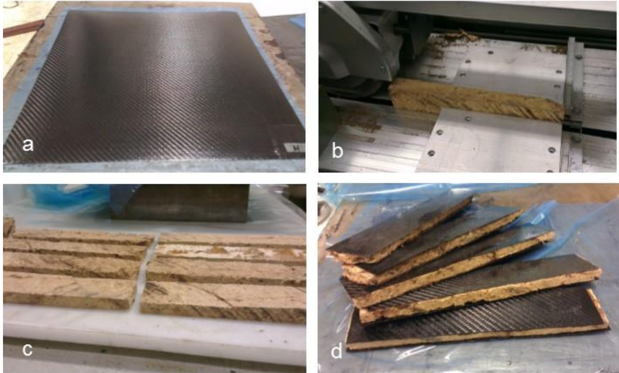
Figure 20. Fabrication of mycelium material sandwich composites with carbon fiber laminate skins (a) 1-ply carbon fiber skin laminate (b) Cutting of mycelium material core (c) Unskinned mycelium composite beam samples (d) Carbon fiber skinned beam samples
