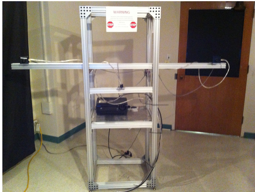
Figure 2.7: A single station in our multi-view structured-light system.
