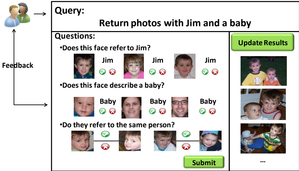
Figure 5.3: User Interface. Given a query, the system will automatically choose some questions to return to users for feedbacks, based on which the query answers will be updated.
