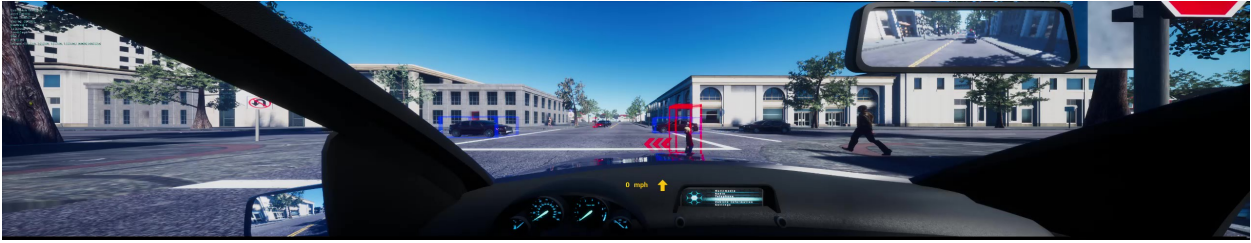
Figure 4.2: This is a forward event intersection with high traffic density, corresponding to the event in Figure 4.6A. We highlight objects using bounding boxes on the user interface: red for pedestrians and blue for cars. In addition, we also display the ego vehicle's current speed and heading direction with yellow texts and arrows in the middle. During the study, this concatenated screenshot is separately shown on three displays to simulate the field-of-view of a driver in the real world (see Figure 4.1).
