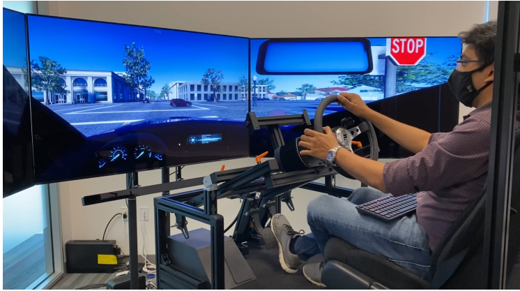
Figure 4.1: Our driving simulator is composed of a steering wheel and two pedals mounted on a cockpit, and three 55-inch displays showing the front and side views of the virtual environment.
