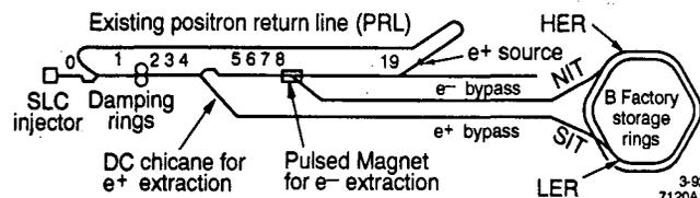
Fig. 1. Schematic of the B Factory e<sup>±</sup> injection system, using the SLC linac and added bypass lines.
