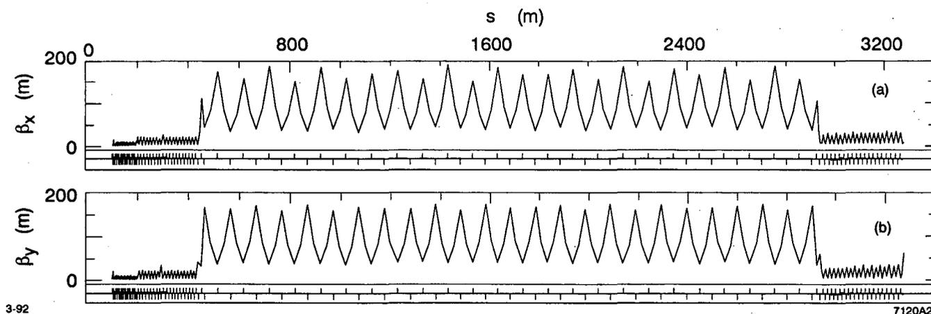
Fig. 2. Optics for the positron extraction, bypass line, connection to SIT and SIT (dispersion not shown).
