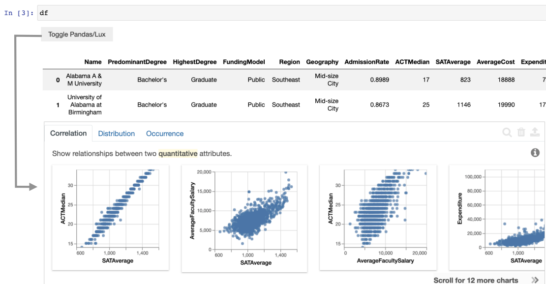
Figure 6.1: Top: When a user prints out a dataframe in LUX, the default pandas table is displayed. Bottom: Users can toggle to browse through a set of dataframe visualizations suggested by LUX.
