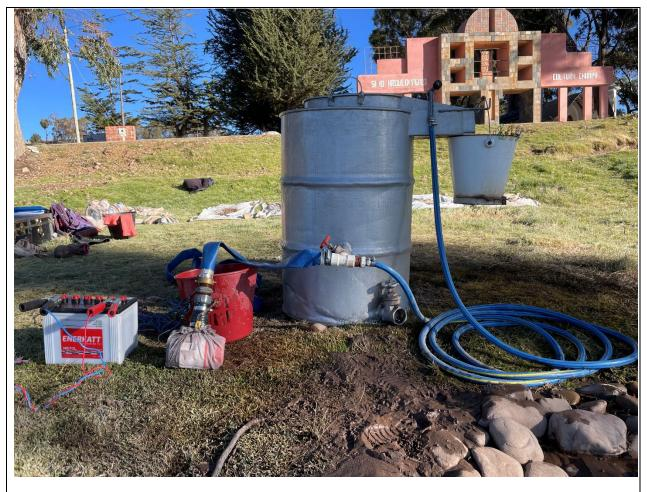
Figure 1. SMAP-style mechanized flotation machine with solar-powered bilge pump used for sample processing.
