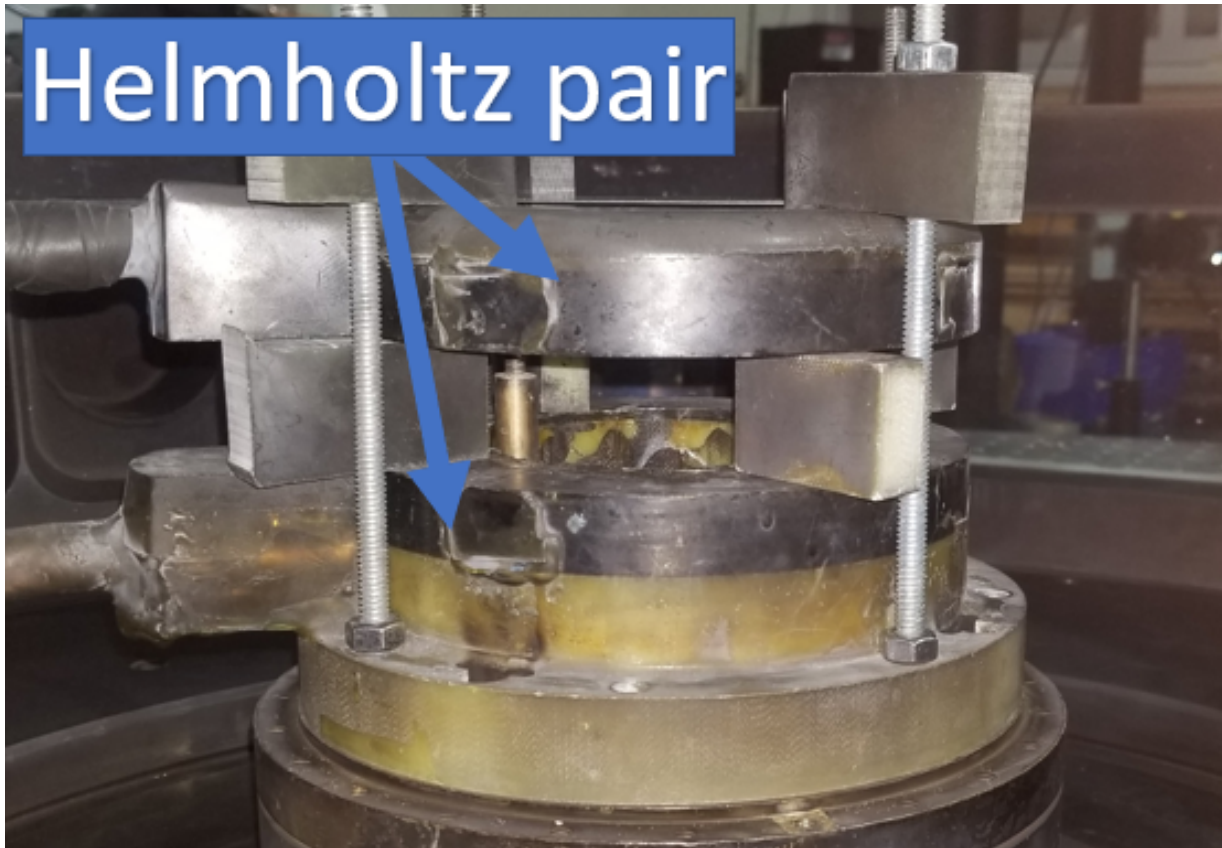
Figure 2.20: Experimental setup for Helmholtz coil pair
