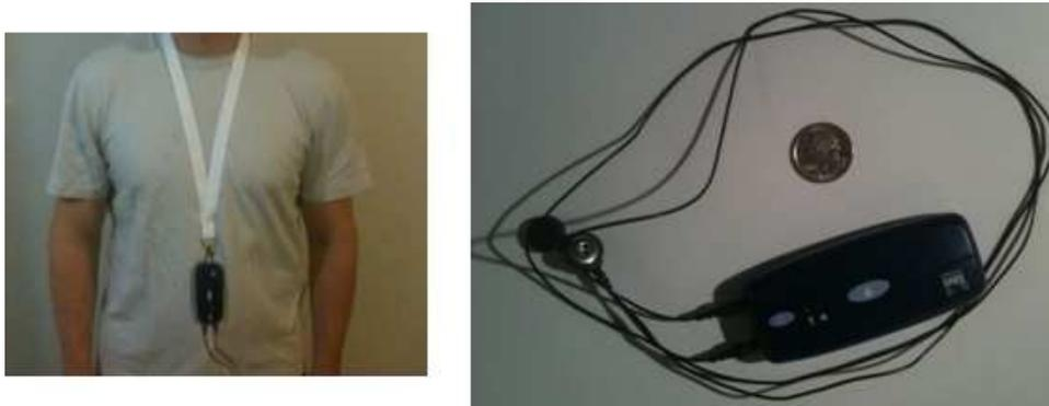
Figure 7.1: Displays the Alive Heart and Activity Monitor by Alive Technologies [Tec12]. The left image shows a subject wearing the device with a lanyard around the neck. The right image shows an up close image of the device with a U.S. quarter for comparison of size.
