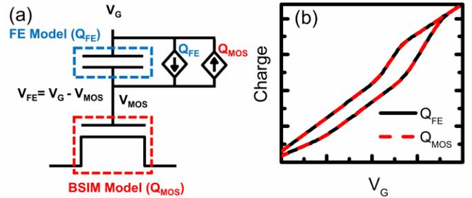
Fig. 1. (a) The equivalent circuit model of FEFET and (b) the charge equality between FE and MOSFET.
